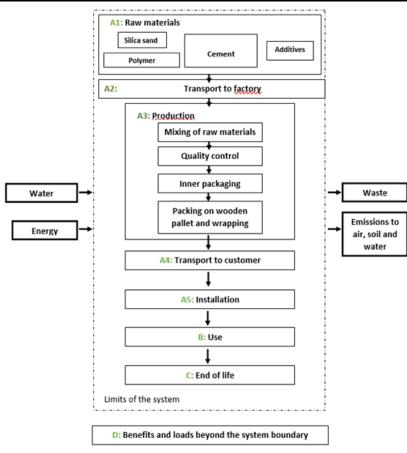
Figure 2: Limits of the system in this study
